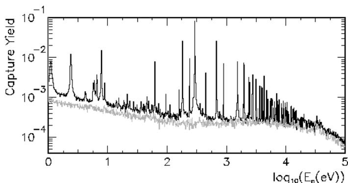
Fig. 1. Capture yield (black) and overall background (grey) for the  $^{91}\text{Zr}$  isotope; most of the resonances up to 150 eV are due to Hf and Sn contamination in the sample.
