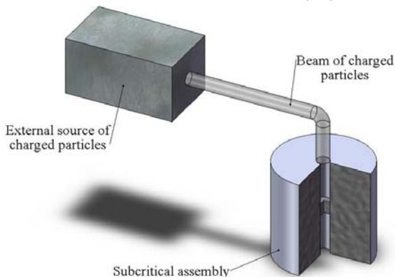
Fig. 1. Simplified scheme of ADS.
