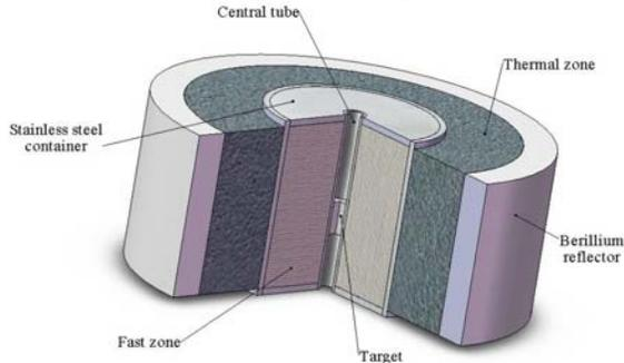
Fig. 2. The simplified sub-critical assembly.
